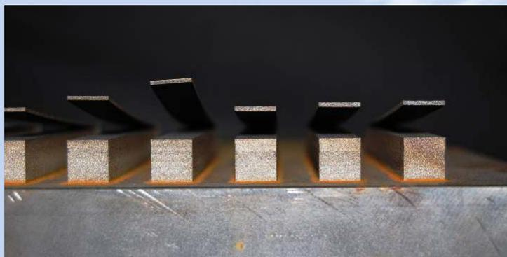
Test bars processed under differing conditions- then the top layer cut to allow residual stress to mechanically relax
