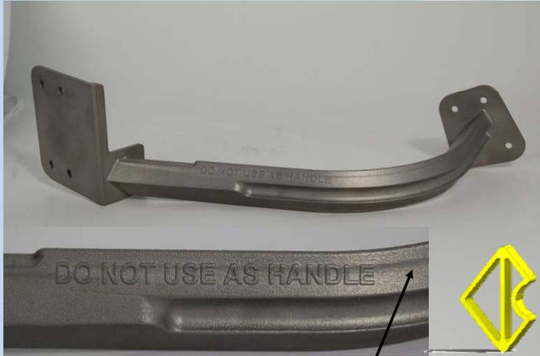
Witness mark geometry related stress driven movement during build
