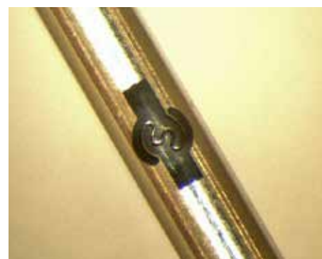
Figure 1: Complex shape machined in 3 materials: nylon, polyimide, nitinol.
