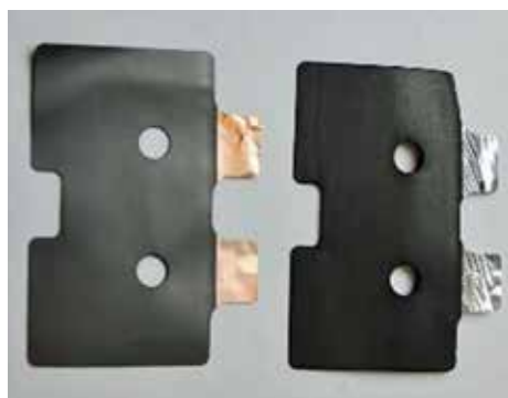
Copper anode and aluminum cathode foils, coated with lithium ion compound.
