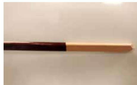
Hairpin ablation of dielectric coating prior to welding.
