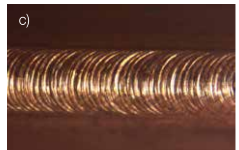
Figure 4: a) Corner weld of 0.5 mm copper sheets, feeding speed 3m/min, b) cross-section view and c) close up weld bead.
