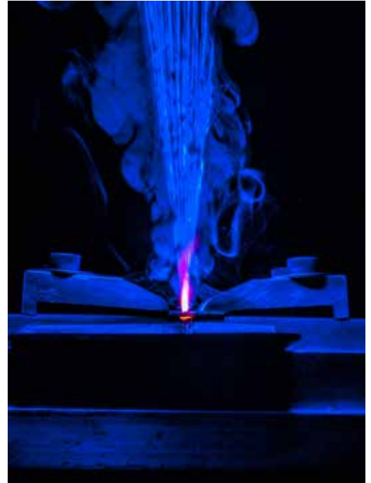
Cover image: A 500 W high power blue laser (AO-500) performing a lap weld of 2 x 300 microns pure copper sheets.
