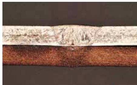
Figure 3: Lap weld of 200 \mu\text{m} -thick copper and stainless steel. This dissimilar materials weld illustrates reduced formation of intermetallics and minimal to no spatter and defects.
