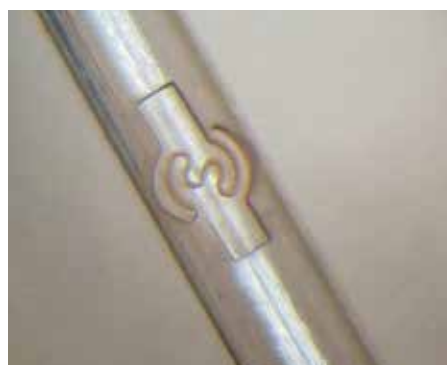
Figure 1: Complex shape machined in 3 materials: nylon, polyimide, nitinol.
