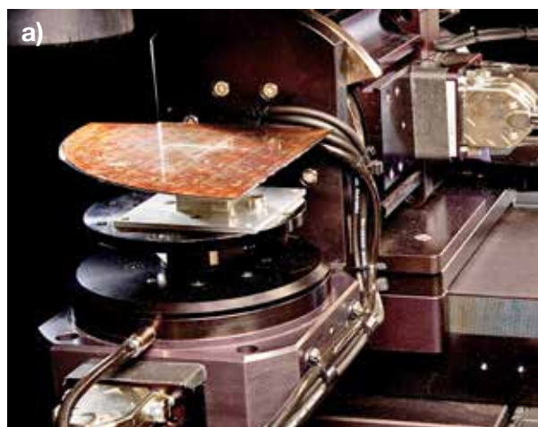
Figure 1: (a) Silicon processing based on Amplitude's Satsuma platform, and incorporating a specific GHz burst source. (b) Typical burst train, with 200 sub pulses at 0.9 GHz repetition rate. Burst total energy 2 mJ. Average power 100 W.
