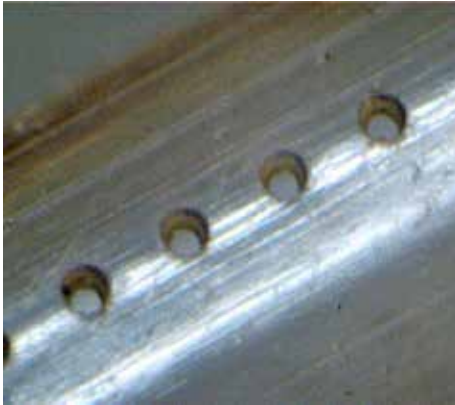
Figure 2: A line of 20um holes in Nylon
