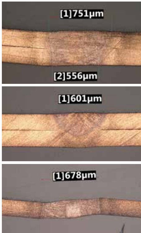
Figure 2: Lap and butt welds illustrate the joint quality routinely achieved with a 500 W blue laser.
