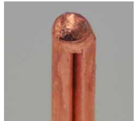
Figure 4: This hairpin weld of two 1.5 mm x 2 mm copper wires demonstrates the quality and compact size possible with blue laser welding.
