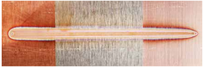
Figure 4: Smooth and extremely stable 450nm laser weld of copper sheet prepared with three different surface conditions (etched, oxidised, polished). Courtesy Laserline GmbH.
