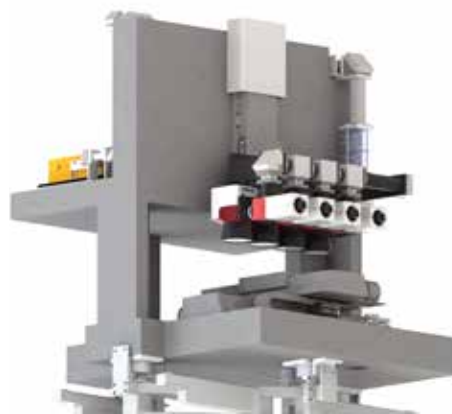
Figure 4: Representation of the design of the final four-head laser machine for a 100 W fs laser.
