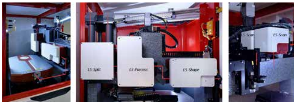
Figure 2: Images of the practical demonstrator built, the back with the Tangor® laser (left); details of the different beam management modules (centre); detail of the two heads galvo from the front (right).
