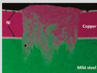
Energy dispersive X-ray analysis showing elements distribution in a fibre laser weld.
