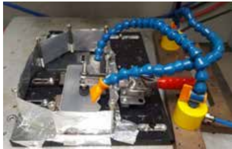
Figure 1: SPI Test station with enclosed bath and argon gas delivery tubes.
