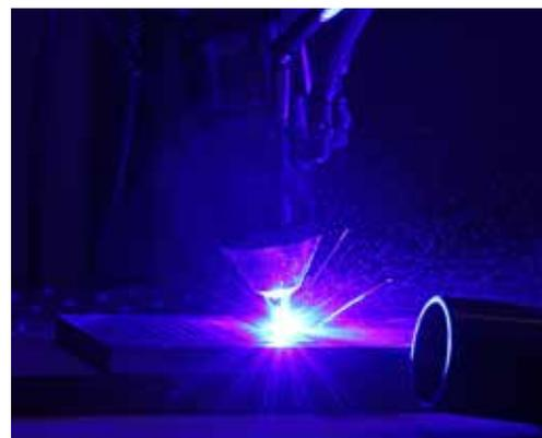
Cover image: A high power diode laser in the blue wavelength (450 nm) performs pore-free cladding (Laser Metal Deposition) with copper powder onto a copper workpiece.
