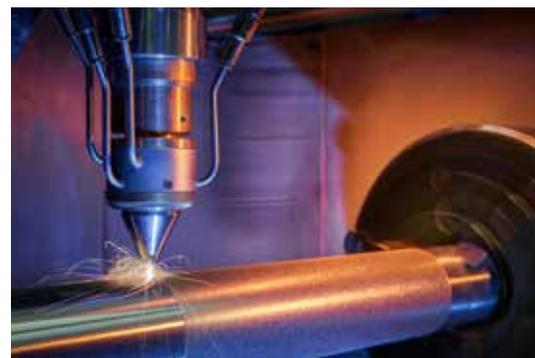
The cover image shows an extreme high-speed laser application (EHLA), where protective metal layers can be applied at extremely high speeds.
