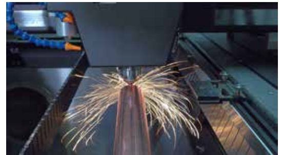
Cover image: Rotary cutting 0.04" stainless steel with a 1.5 kW fibre laser at 125 in/min.
