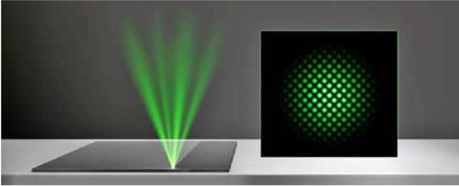
Figure 3: (left) Superposition of four partial beams from the same laser source to form a dot-like interference pattern (right). © Fusion Bionic
