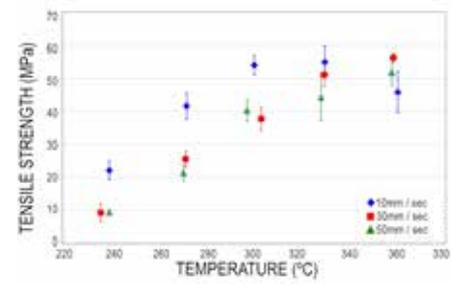
Figure 5: Relationship between the processing point temperature and welding strength
