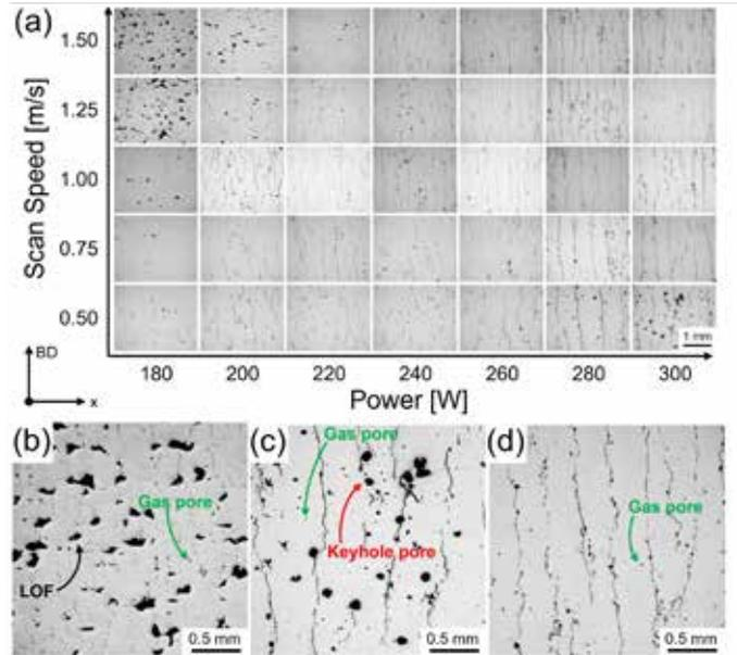
**Figure 4:** (a) Optical micrographs of all the P-v combinations experimentally investigated within the optimised process window; (b) Typical microstructure of a sample in the LOF region; (c) Microstructure obtained in P-v combinations predicting the presence of keyhole pores; (d) Typical microstructure of a sample in the gas pores area.
