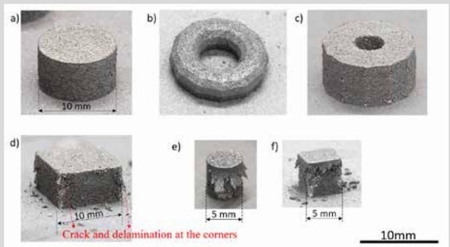
*Figure 1: Printed demonstrators showing the design freedom capabilities and limitations when using laser powder bed fusion to process NdFeB magnets*
