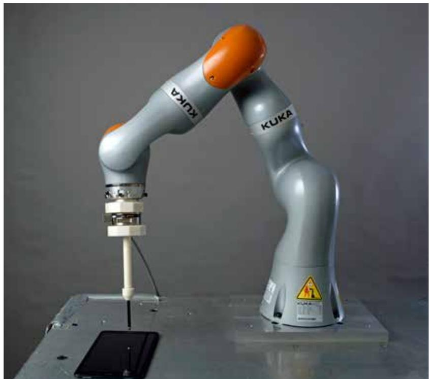
*Figure 4: Example robotic manipulator (arm). This Kuka robot is of the order of 1 m with a reach and load capacity to cover a typical laser build bed. With accuracies in the order of ~1mm it can replicate a human alignment process given the right programming.*
