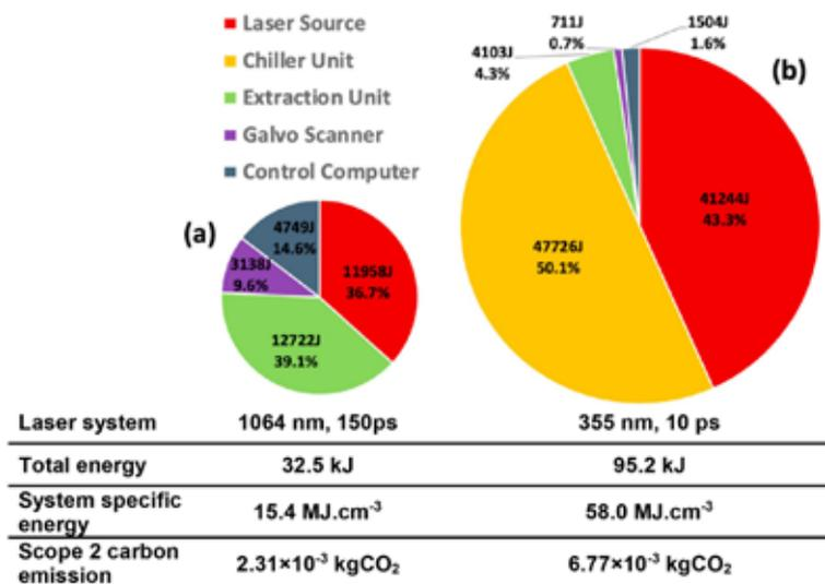
Figure 1: Sub-system energy comparison for laser cleaning of a tool insert using a) IPG 1064 nm, 150 ps, and b) EdgeWave 355nm, 10 ps laser systems [4]
