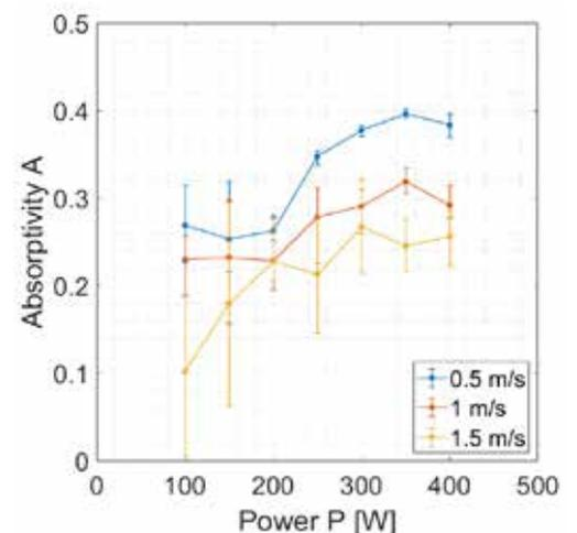
Figure 2: Laser absorptivity of AA2024 powders during L-PBF as a function of laser power and scan speed.
