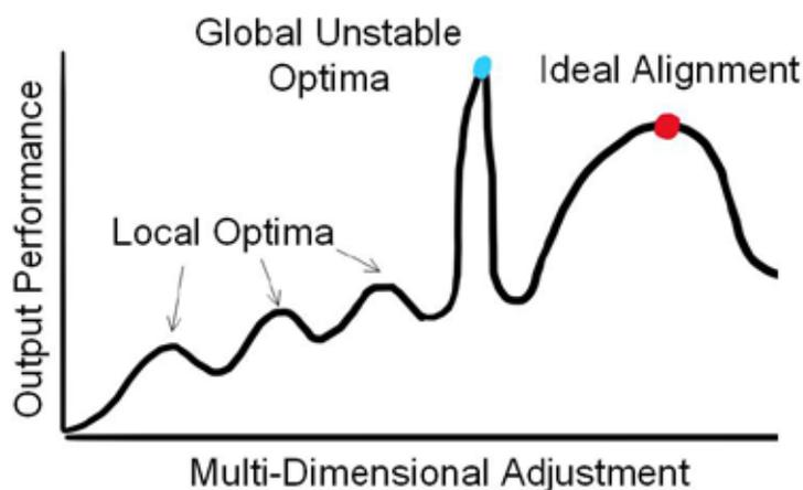
*Figure 1: Graphical illustration of a complex alignment space. Complex multi-dimensional spaces of this sort are typical of laser systems. In this case the system exhibits a number of local optima as well as an unstable global maxima which would be avoided in comparison to the more stable ideal position.*
