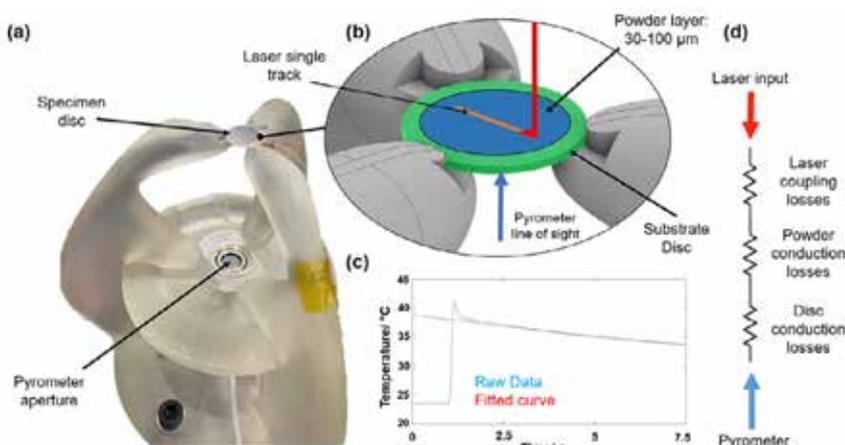
Figure 1: (a) Overview of the laser calorimetry system used to measure the absorptivity of AA2024 powders during L-PBF; (b) Detail of the disc's holding mechanism; (c) Curve fitting from raw data to evaluate temperature decrease over time; more information about this calorimetry system can be found in [5].
