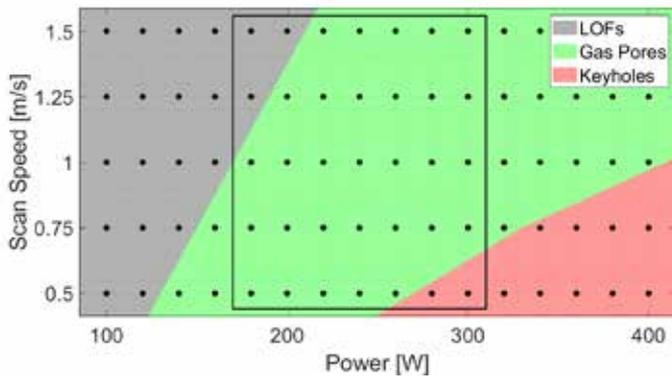
**Figure 3:** Graphical output of the prediction of the presence of LOFs (grey region), keyholes (red region) and gas pores (green region). The refined process window is enclosed by the black box.
