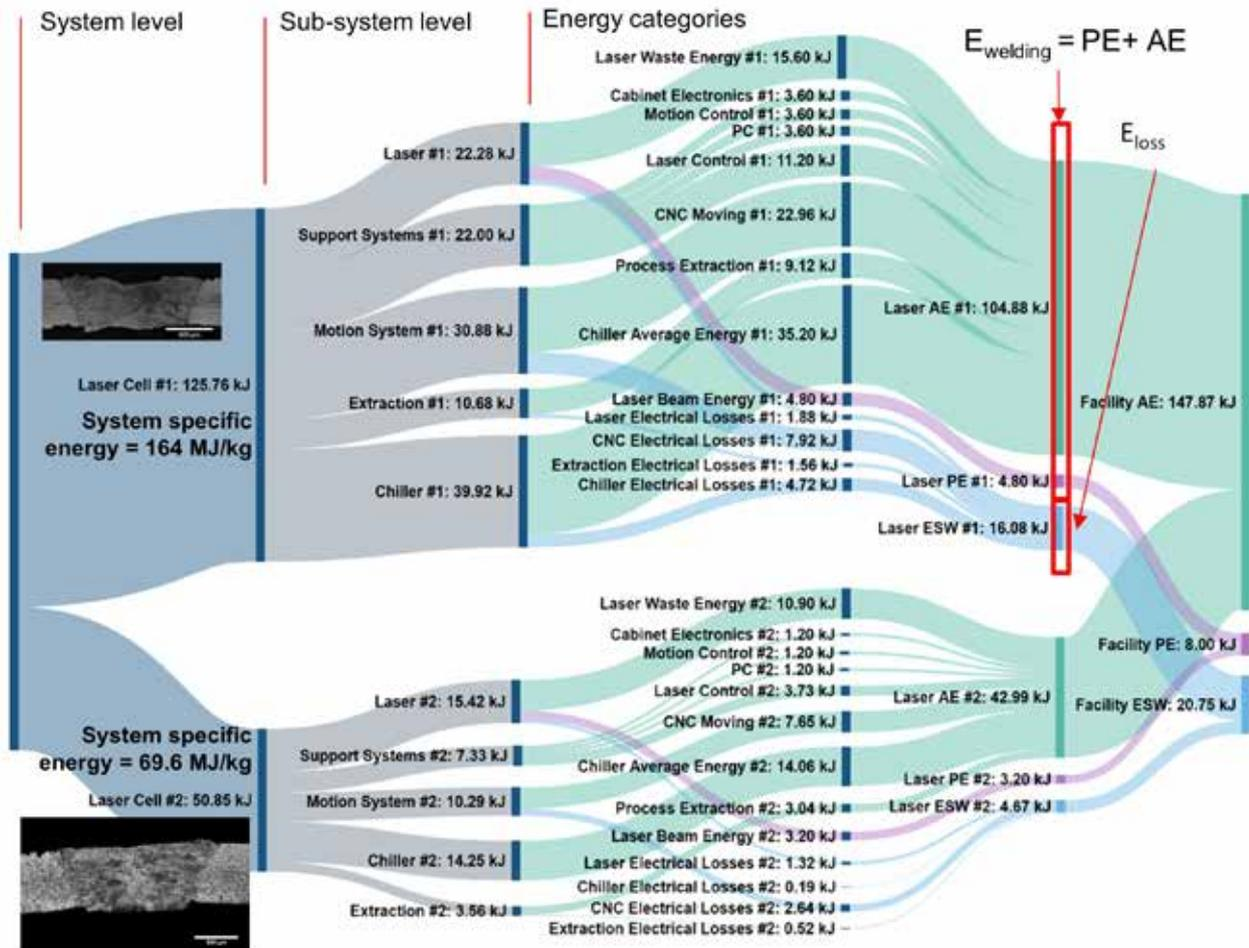
Figure 2: Sankey diagram showing the breakdown of energy categories and the energy use for two welding production cells using a 300 W, 1070 nm fibre laser [5].
