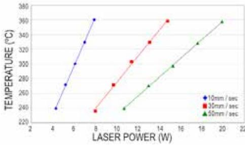
Figure 3: The relationship between power and temperature at different processing speeds
