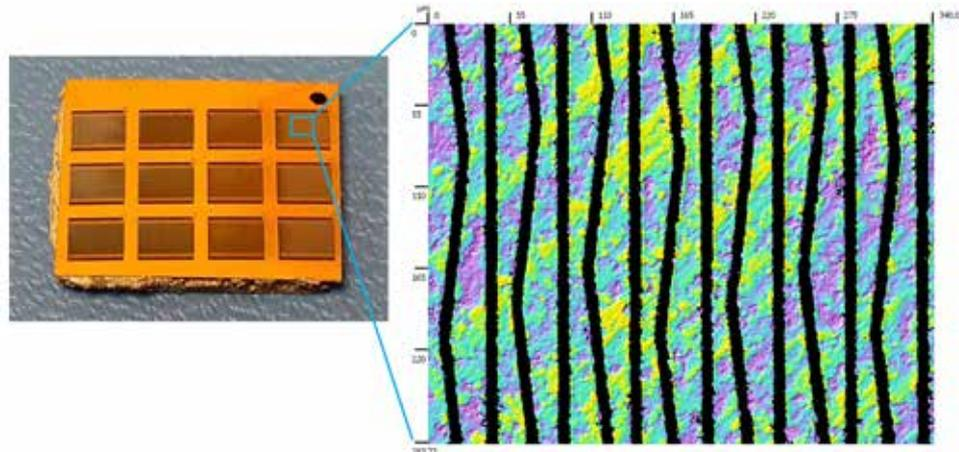
Figure 2: Photograph of an acoustic panel showing 12 individual arrays directly after laser processing at OL (left) and confocal microscope image of the resulting cut elements (right).
