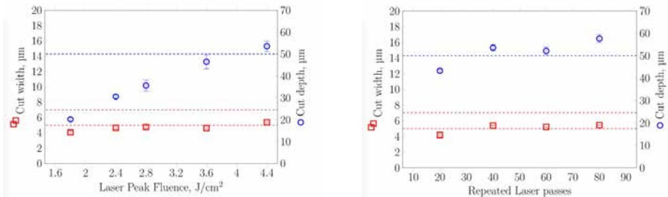
Figure 1: Single beam process development. Moderate fluences and many passes are required for achieving precise element singulation of 50  $\mu\text{m}$  thick PZT substrates with cut street width below 8  $\mu\text{m}$ .
