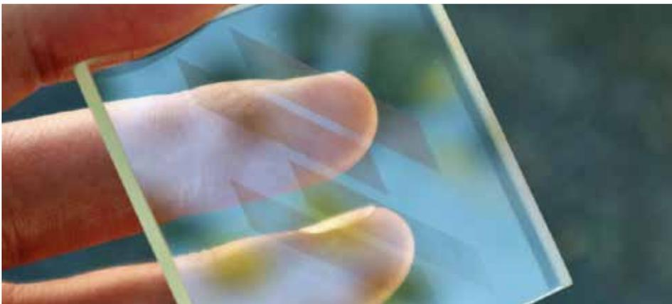
Figure 5: Glass substrate textured with DLIP for anti-reflection. The periodic structures inscribed on the glass and forming the Fusion Bionic's logo mimic the moth-eye structures and reduce the amount of reflected sunlight. © Fusion Bionic
