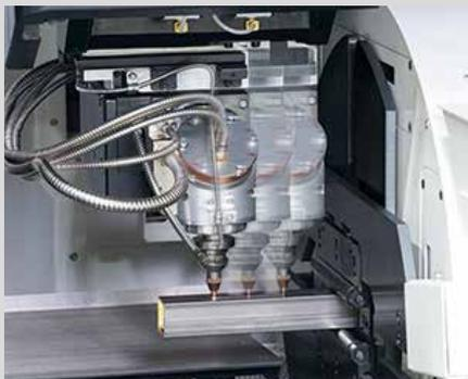
The FT-150 FIBER from Mazak is its latest laser tube processing machine specifically designed for the high-speed cutting of small and medium tubes up to 152.4mm diameter in large-lot and for high productivity.
