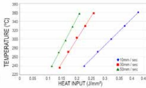
Figure 4: The relationship between heat input and temperature at different processing speeds
