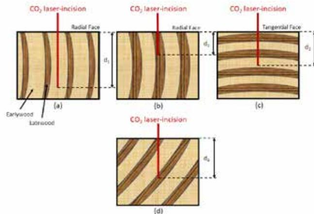
*Figure 1: Schematic diagrams of CO<sub>2</sub> laser-incision strategies with CO<sub>2</sub> laser interaction with earlywood and latewood tissues in the structure of wood.*
