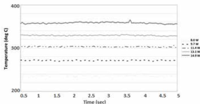
Figure 2: Measurement temperature at the time of laser welding when scanning at 30 mm/sec.
