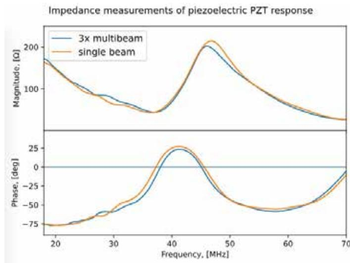
Figure 3: Impedance measurements of multi vs single-beam processing showing identical piezoelectric response directly after laser processing. Introducing a multi-beam approach speeds up the process without compromising the high-frequency piezoelectric response at around 40 MHz.
