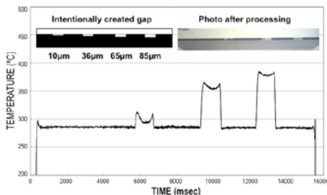
Figure 6: Experimental results of gap detection
