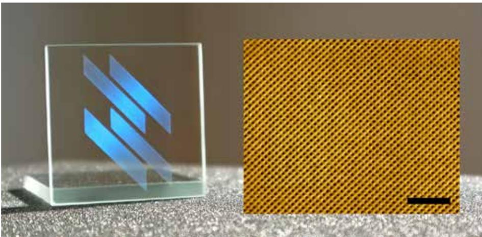
Figure 4: (left) Glass substrate textured with DLIP, showing a blue Fusion Bionic's logo and (right) microscope image of the surface structures inscribed on the glass surface responsible of the structural colours (scalebar: 10 µm). © Fusion Bionic
