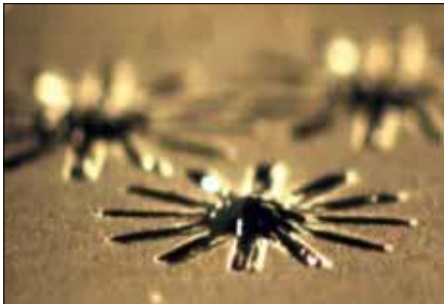
Figure 2. Surfi-Sculpt feature made in polypropylene using a few Watts of CO 2 laser radiation.
