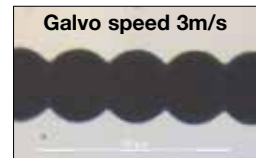
Figure 3. 1064 nm scribing of 20 nm aluminum on glass Galvo speed 4m/s Galvo speed 3m/s
