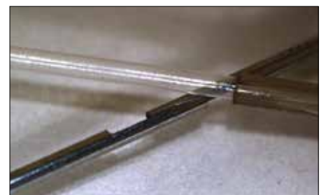
Figure 2: 'Stop on layer' stripping of 0.1 mm polymer lining from a PTFE tube of wall thickness 0.025 mm without residual damage. (Courtesy Blueacre Technology)
