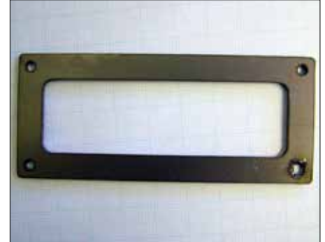
Figure 2: Small detail burning in thin mild steel when cutting with too much laser power.
