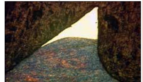
Saw-tooth tip selectively hardened using an HPDDL
