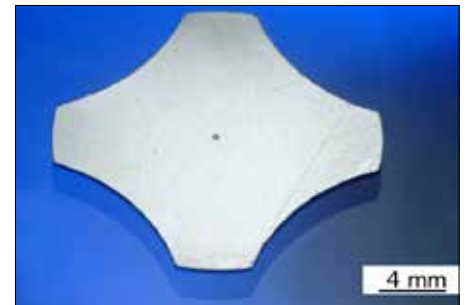
Figure 8: A switch with a silver contact made by laser micro-cladding
