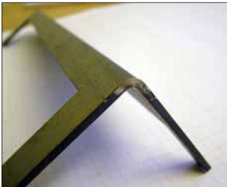
Figure 1: A 3 mm thick mild steel item cut with oxygen assistance and subsequently bent. Note: the flaking off of the oxide layer on the cut edge in the area where the bend took place.
