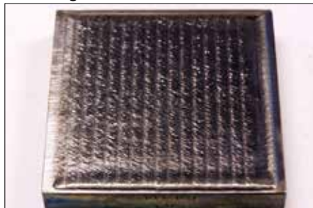
Multi-pass clad of NiCr powder material resulting in a clad 1.5 mm thick on 1018 steel plate. The clad rate was 0.45 m/min at 4 kW laser power
