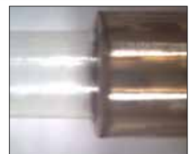
Figure 2: 'Stop on layer' stripping of 0.1 mm polymer lining from a PTFE tube of wall thickness 0.025 mm without residual damage. (Courtesy Blueacre Technology)
