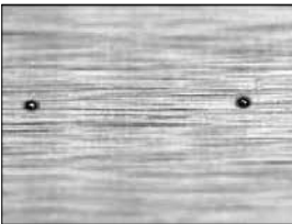
Figure 9: Fuel cell collector plate with gold contacts (Courtesy FZ Jülich)
