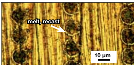
Figure 1: Copper ablation with single laser pulses (1ns, 10 \mu\text{J} ) focused to a 10 \mu\text{m} diameter spot
