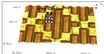
Figure 11: Ablated cell with cross-scan produced in copper, depth 25 \mu\text{m}
