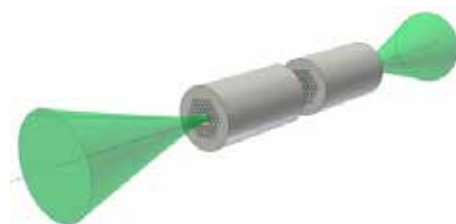
Figure 2a: Beam propagation through a micro-structured hollow core fibre
