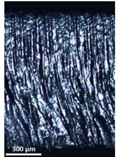
Figure 1: Cut edge of the 1.2 mm thick AA2024 aluminium alloy processed using 68 kW/mm 2 of power density and a travel speed of 120 mm/s
