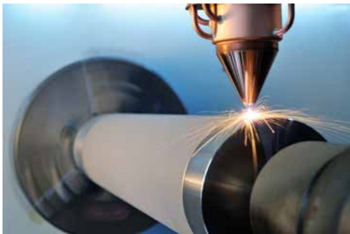
Figure 2: Coating of a hydraulic plunger with ultra-high speed laser cladding (source: Fraunhofer ILT)
