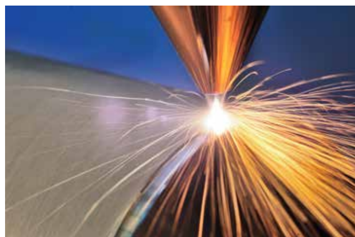
Figure 2: Coating of a hydraulic plunger with ultra-high speed laser cladding (source: Fraunhofer ILT)
