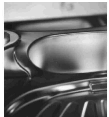
Figure 3. Welding a kitchen sink with a high power diode laser. (left) positioning the laser head in a robot, (right) kitchen sink after welding.
