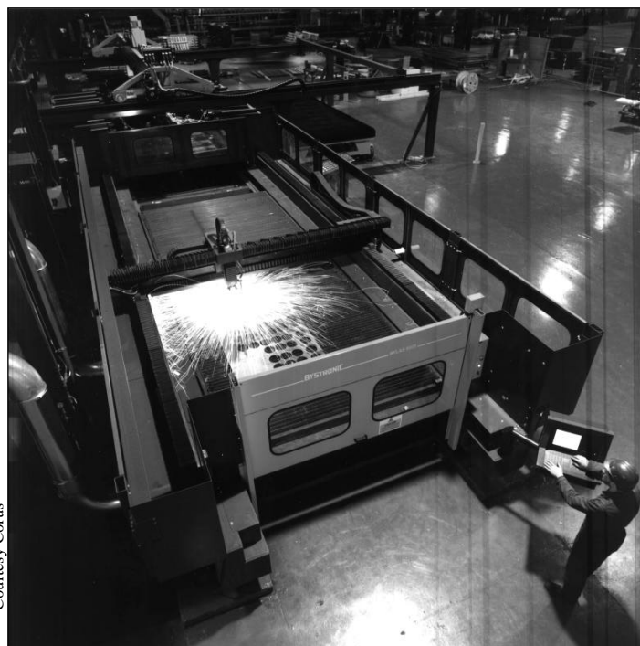
Figure 1. An open-topped flatbed CO 2 laser cutting machine with guarding providing full peripheral protection.
