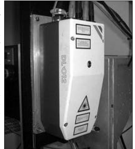
Diode laser head on a rig at the IMC, University of Warwick.
