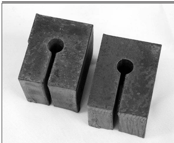
Figure 4. LASOX cuts showing 10 mm diameter holes in 40 mm plate.
