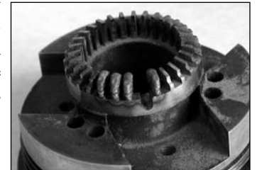
Worn tooth repair by laser cladding
