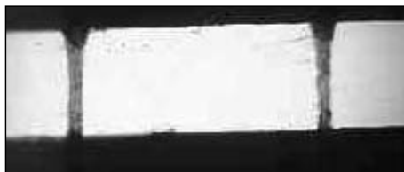
10 \mu m diameter holes drilled in a 50 m thick stainless steel sheet using an ultra-fast laser
