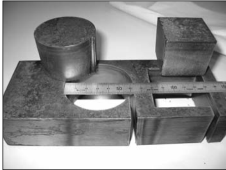
Profile cut obtained in 40 mm thick, 250 grade mild steel plate with a Nd:YAG laser power of 2 kW.
