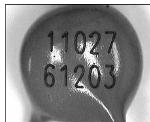
2mm-high text marked on an electrical component
