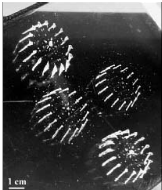
Figure 4. Picture of a PMMA sample microstructured with a CO 2 -laser together with a diamond fan-out element. The picture shows four different exposures (exposure time 0.5 s) with slightly varying distance between the DOE and PMMA sample. The patterns at the top left and bottom right are non-optimal due to a slight tilting of the DOE during exposure.
