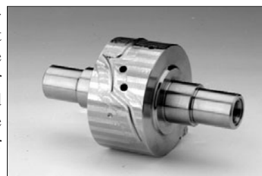
Fig 3. Repair of a cutting roller: (top) cutting roller after two layer coating (bottom) after reworking by a machining process to produce a new blade.
