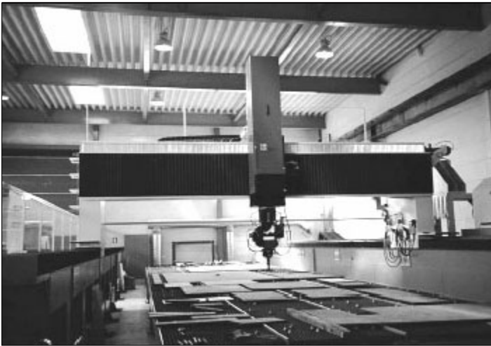
Figure 3: The 12kW CO 2 laser cutting and welding test facility at Odense Steel Shipyard in Denmark
