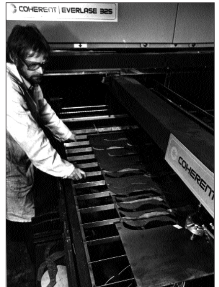
Newspaper clipping from May 1979. Lasercut Product's general manager, Brian Sandford watches the progress of a 'computer controlled roving nozzle' on the UK's first industrial laser machine with moving optics.
