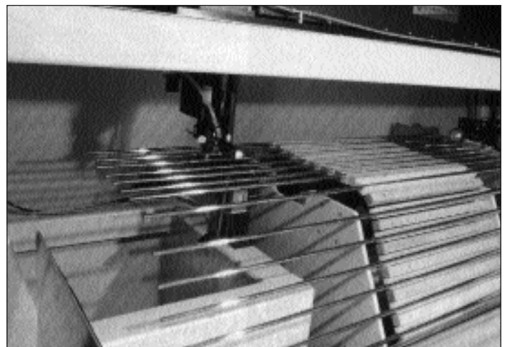
Figure 2. Sealed-tube CO 2 laser cutting golf-club shafts.
