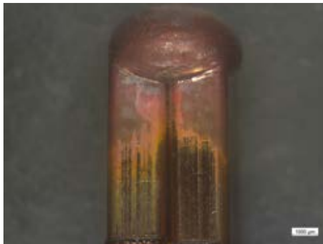
Figure 1: Welding of copper hairpins with a cross-section of 9.9 mm 2 each in approximately 250 ms. ©Laserline
