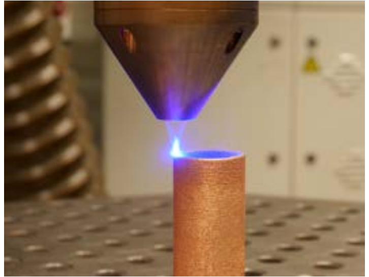
Figure 3: Additive Manufacturing using copper powder by directed energy deposition and a blue diode laser ©Laserline
