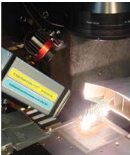
Figure 1: Monitoring of USPL induced X-ray photon emissions by using the X-ray Guard SILIX.
