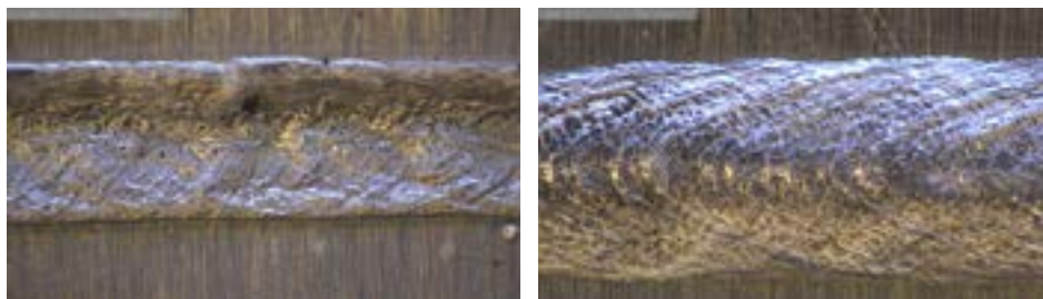
Figure 1: Examination of the surface of the welds achieved without ultrasound (left) and with ultrasound (right).
