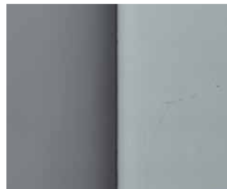
Figure 2: PLA sheet after dicing and fracture showing the smooth cut edge.
