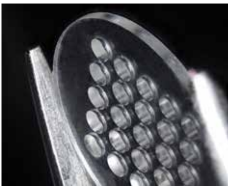
Figure 4: An example shape cut from biodegradable polymer using ultrashort pulses. The diameter of the holes is 500 \mu\text{m} .
